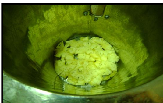
Fluidized bed drying of pineapple slices
