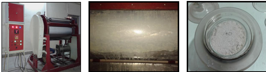
Plate 2: Drum drying of peanut milk
