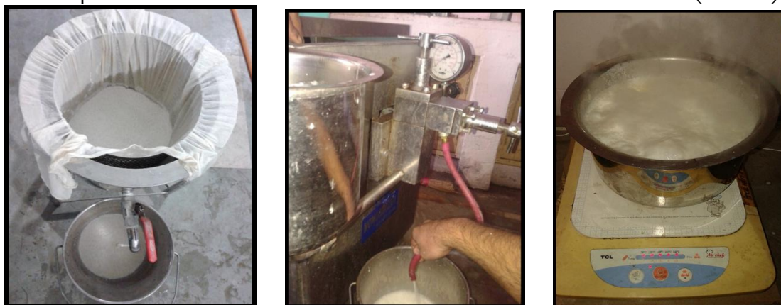
Plate 1: Filtration, homogenization and pasteurization of peanut milk.
