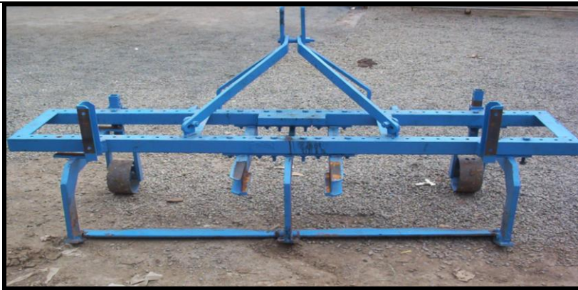
Fig. 1: Existing Tractor Drawn Groundnut Digger with Depth Control Wheels
