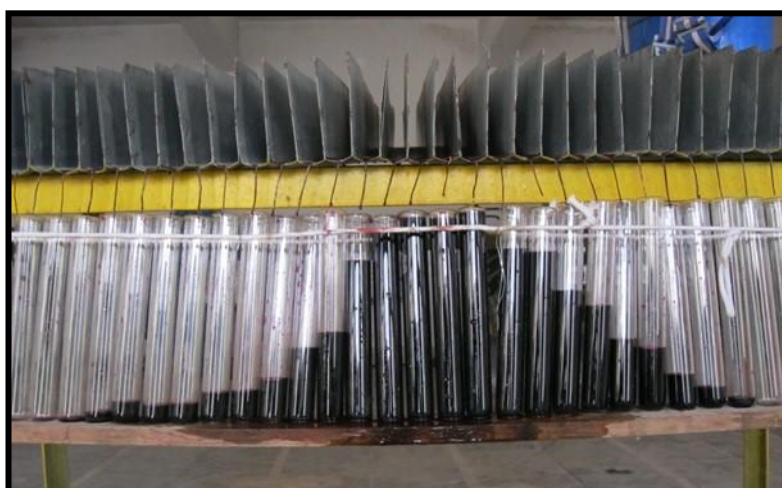
Fig. 8: Testing of single nozzle spray lance on patternator
