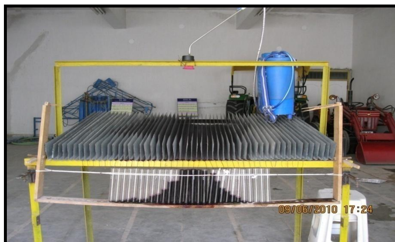
Fig. 6: Set up of spray patternator for nozzle testing
