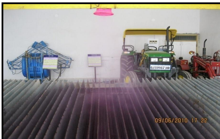
Fig. 7: Spraying of KMNO_4 solution on patternator
